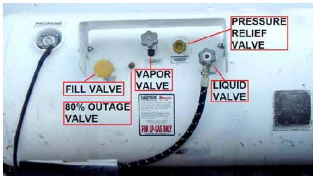
Figure 9. Propane autogas fuel tank
