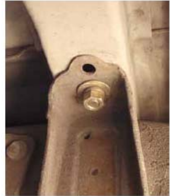
Figure 18. Bed-mount installation that also serves as a tank mount
