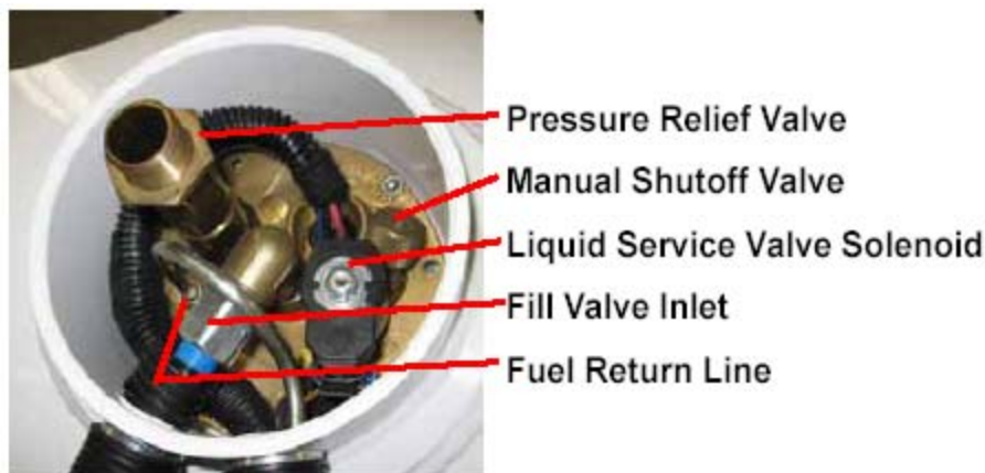
Figure 10. LPI tank valves. The valves are located under the access plate. See Figure 11.
