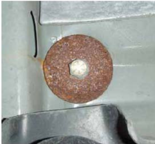
Figure19. Load-spreading washer located under vehicle bed
