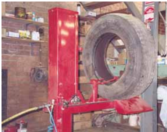
Low risk example. Bead breaker and mechanical aid used with leak detection bath.
